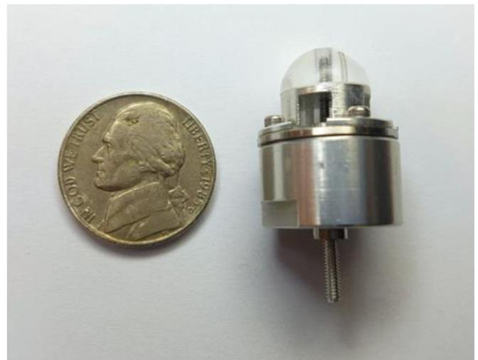
Fig. 8. Fabricated micro-tattooing device with US five-cent coin (Prototype).
