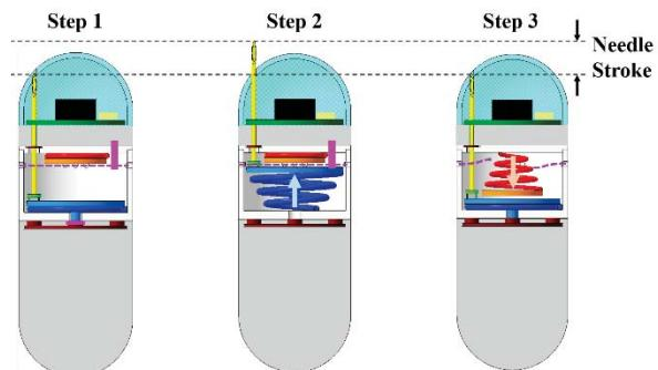
Fig. 2. Working principle of tattooing module.
