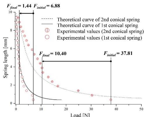
Fig. 3. Experimental data of conical springs.
