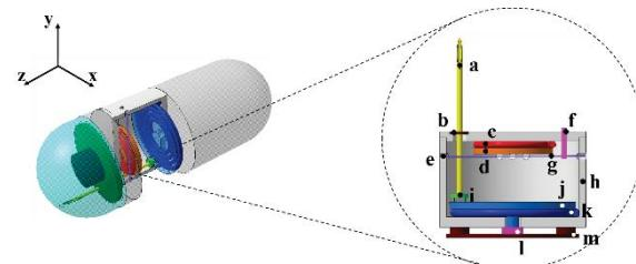
Fig. 1. Configuration of tattooing module: a. Needle, b. Rubber stopper, c. 2nd conical spring, d. Plate, e. Nylon cable hole, f. SMA wire, g. Nylon cable, h. Housing, i. Needle holder, j. Acrylic post, k. 1st conical spring, l. Ni-Cr wire, m. Heat shield
