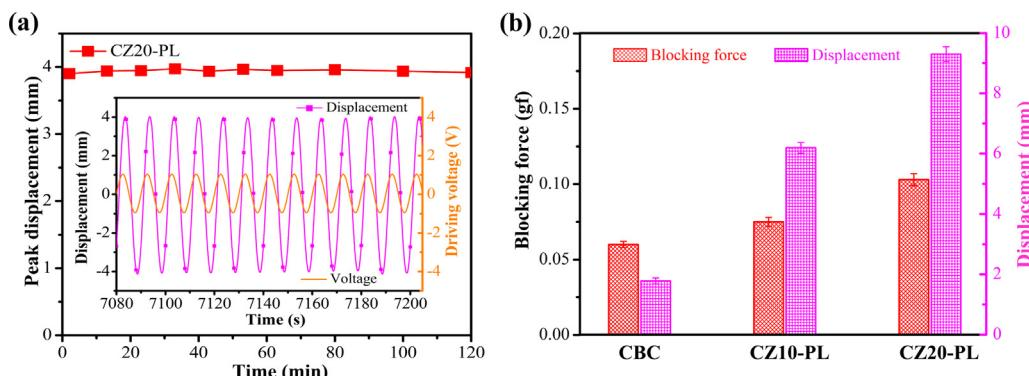
**Fig. 9.** (a) Actuation durability of the CZ20-PL muscular actuator under a sinusoidal excitation of 1.0 V at 0.1 Hz, (b) blocking force of the CBC and CZ20-PL actuator.
