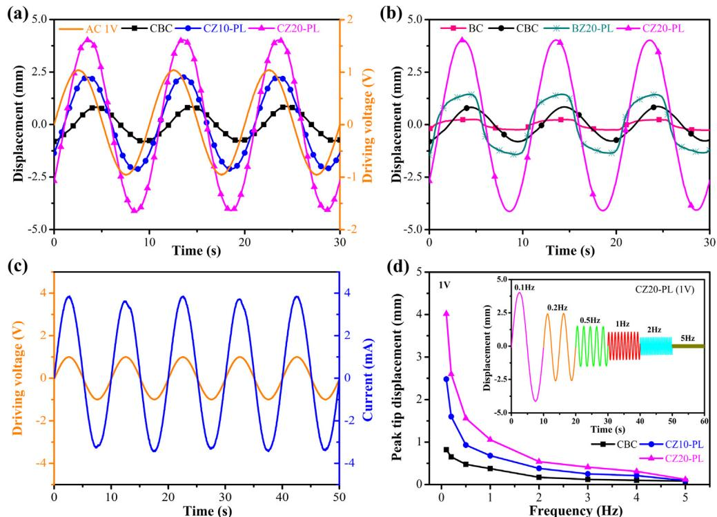
Fig. 6. Actuation performances of the CZ-PL muscular actuators: (a) harmonic responses under a sinusoidal excitation of 1.0V at 0.1 Hz, (b) harmonic responses of the BC and BZ20-PL actuator under 1.0V at 0.1 Hz, (c) current responses, (d) peak displacement under various frequencies.
