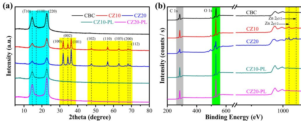
**Fig. 3.** (a) XRD curves and (b) XPS spectra of the pure CBC, CZ, and CZ-PL membranes.
