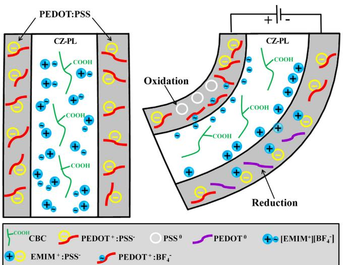
**Fig. 1.** Illustration of the actuation mechanism of the CZ-PL muscular actuator.
