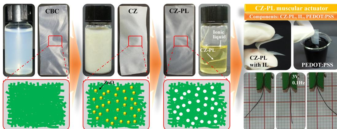
**Scheme 1.** Fabrication of the CZ-PL muscular actuator with the nonmetallic flexible PEDOT:PSS as an electrode.
