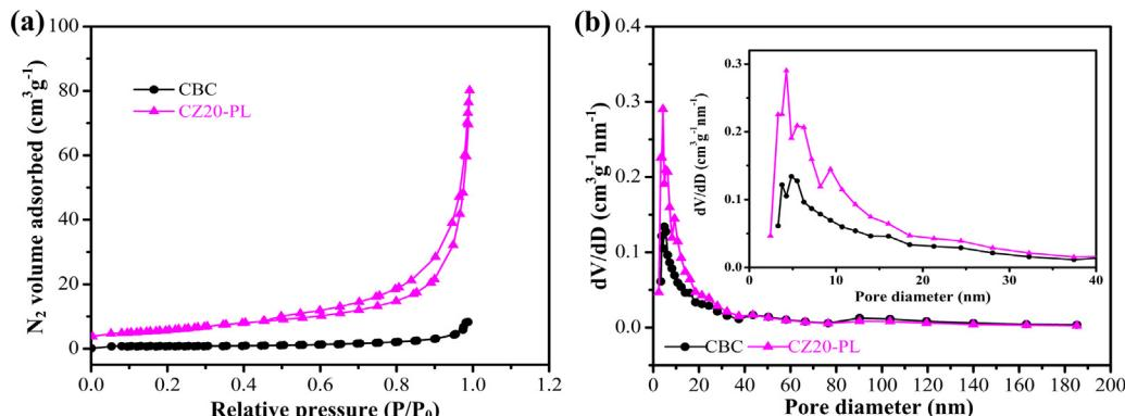
**Fig. 4.** (a) N<sub>2</sub> adsorption-desorption isotherms of the pure CBC and CZ20-PL membranes, (b) pore size distribution for the pure CBC and CZ20-PL membranes at 0–200 nm and 0–40 nm.
