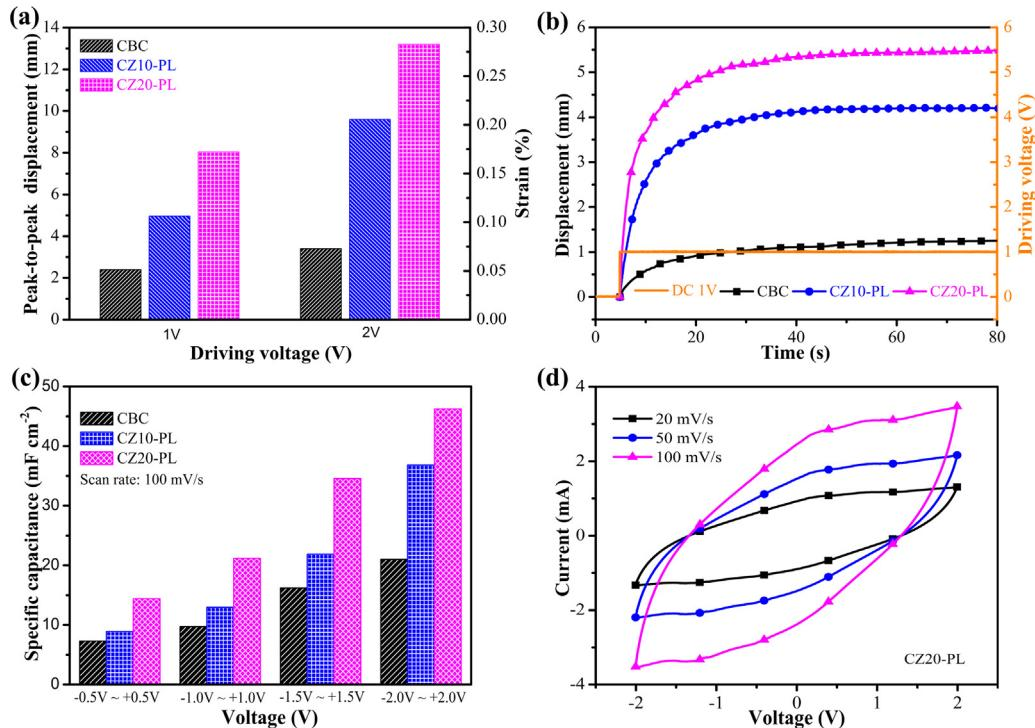
**Fig. 7.** (a) peak-to-peak displacement at different voltages and (b) step responses of the CZ-PL actuator, (c) specific capacitance of the CZ-PL actuator under various voltages at a scan rate of 100 mV s<sup>-1</sup>, and (d) CV curves of the CZ-PL actuator under different scan rates.
