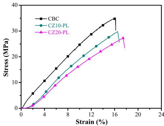
Fig. 5. Stress-strain curves of the pure CBC, CZ10-PL, and CZ20-PL membranes.
