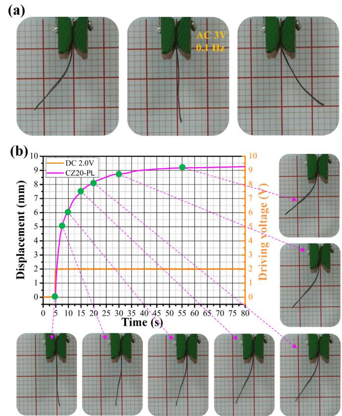
**Fig. 8.** Electromechanically deformed shapes of the CZ20-PL muscular actuator under (a) a sinusoidal excitation of 3.0 V at 0.1 Hz and (b) a step excitation of 2.0 V.
