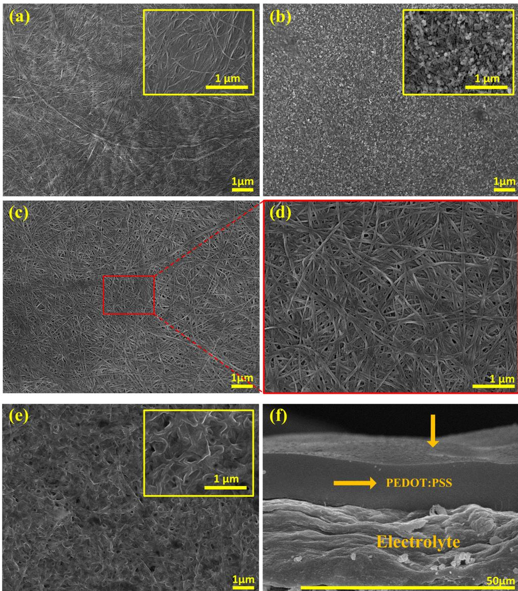
**Fig. 2.** FE-SEM images: (a–c) surface images of the pure CBC, CZ20, and CZ20-PL membranes, (d) magnified surface image of the CZ20-PL membrane, (e) surface image of the CZ20-PL membrane with ionic liquid, (f) cross-sectional image of the CZ20-PL muscular actuator.
